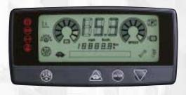
The combination of LED displays and 7-digit graphic LCD display intelligently provides operators with all the details they need, including operational information, diagnostics, and programmable settings. The 4 display buttons offers a choice of four power modes; heavy duty, standard duty, economic duty and slow travel speed mode. Standard instrument images are displayed at the right.
