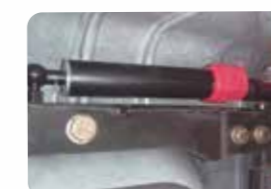
Locking type gas spring
